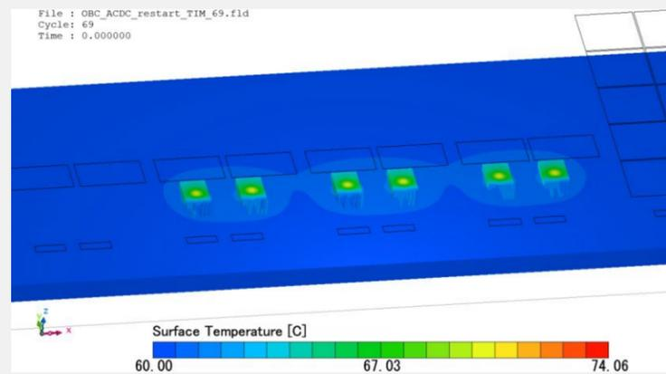
Temperature on the chip area of the MOSFETs
