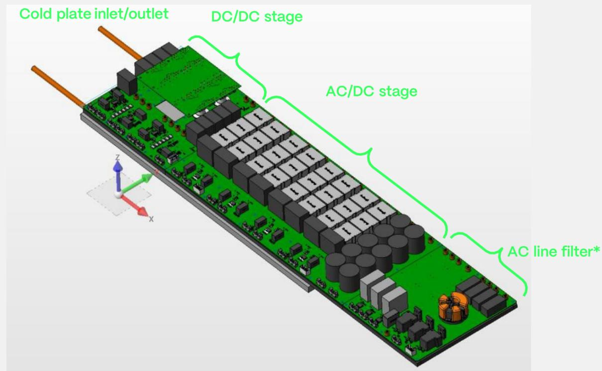
\*For the first prototype, 3 separate PCBs were designed and manufactured for the 3 OBC stages.
